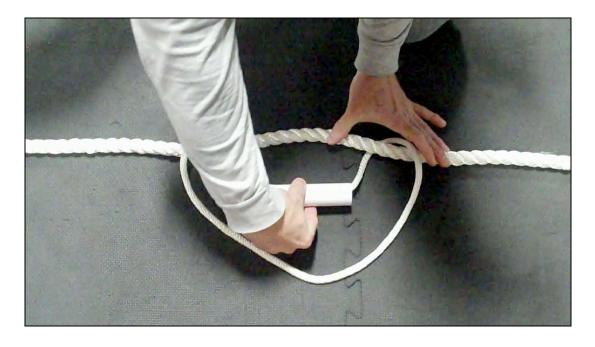
Then take the 'pipe-side' of the loop underneath the main rope and pull it on through the other side of the loop.
