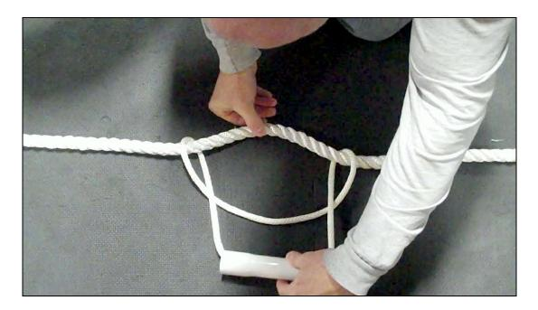
The next step is to take the 'pipe-side' of the loop around the main rope one more time, the very same way that you did the first time. (This is why you don't pull the loop 'tight' around the main rope after making the first loop.)
