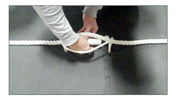
You are now ready to begin pulling the loop tight in order to form the finished knot. As you begin pulling on the loop, use your other hand to start sliding the outside ends of the knot together as shown in the photo below.
